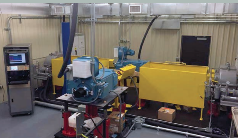
TARDEC's axle efficiency test stand is used in the development of Fuel Efficient Gear Oil. (U.S. Army photo)
