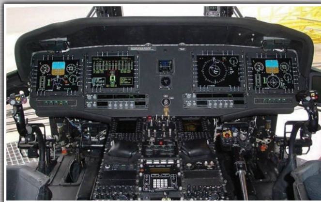
FROM TOP: The electronic instrument displays found in the newest variants of the UH-60 Black Hawk will help extend the life and capabilities of the helicopter. (Photo courtesy of Northrop Grumman)
