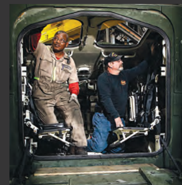
Employees from Anniston Army Depot and General Dynamics Land Systems work on the Stryker Double-V Hull (DVH) Exchange program. Responding to an Army requirement for additional DVH vehicles and to reduce overall vehicle cost, the program changes the hull of a flat-bottom Stryker for the newer DVH design. (U.S. Army photos by Mark Cleghorn)
