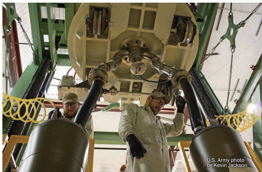
Heath Eldridge, left, and Brad Cochran monitor the transfer of explosives into the body of a BLU-109 C/B penetrator bomb during first article acceptance testing at MCAAP. The 600-gallon mixing bowl rolls on a track to the back of the new B-Line facility and is then elevated for the mix to be transferred into the bomb body that is secured below.
