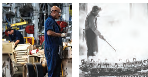
FRONT COVER: Anniston Army Depot employees disassemble M1 Abrams tanks in the Combat Vehicle Repair Facility. The depot is capable of overhauling, repairing or resetting any variant of the M1, to include the Assault Breacher Vehicle and bridging systems supported by the M1 chassis.
