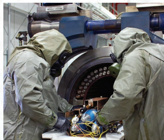
The Explosive Destruction System can treat up to six chemical warfare materiel items simultaneously on-site. The transportable system contains all blast, vapor and metal fragments – protecting the surrounding environment and the system operators. (U.S. Army photo)
