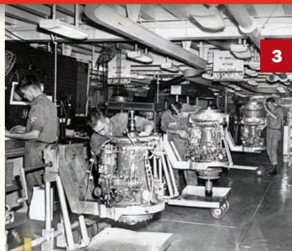
Aboard the USNS Corpus Christi Bay: 1. Four rotor blades are worked on in the maintenance area. 2. A UH-1 belonging to 1st Transportation Battalion is tied down to deck. 3. Soldiers work in an engine test cell in Vietnam. (U.S. Army photos)
