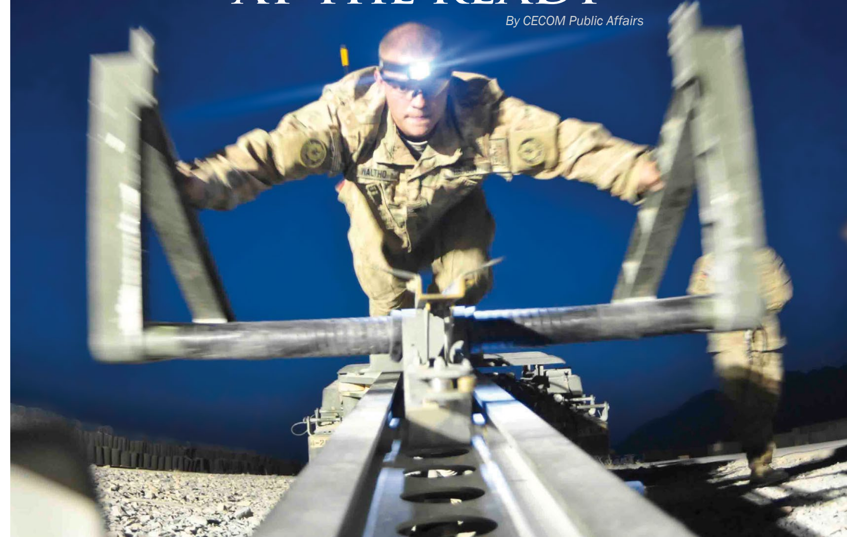
Spc. Justin Waltho, Headquarters and Headquarters Troop, Combined Task Force Dragoon, resets a launcher for an RQ7B Shadow Technical Unmanned Aircraft System at Forward Operating Base Pasab, in Kandahar Province, Afghanistan. The aircraft was used for aerial reconnaissance and mission communications. CECOM services a variety of reconnaissance and mission communications systems to enable Soldier dominance on the battlefield. (U.S. Army photo by Sgt. Joshua Edwards)
