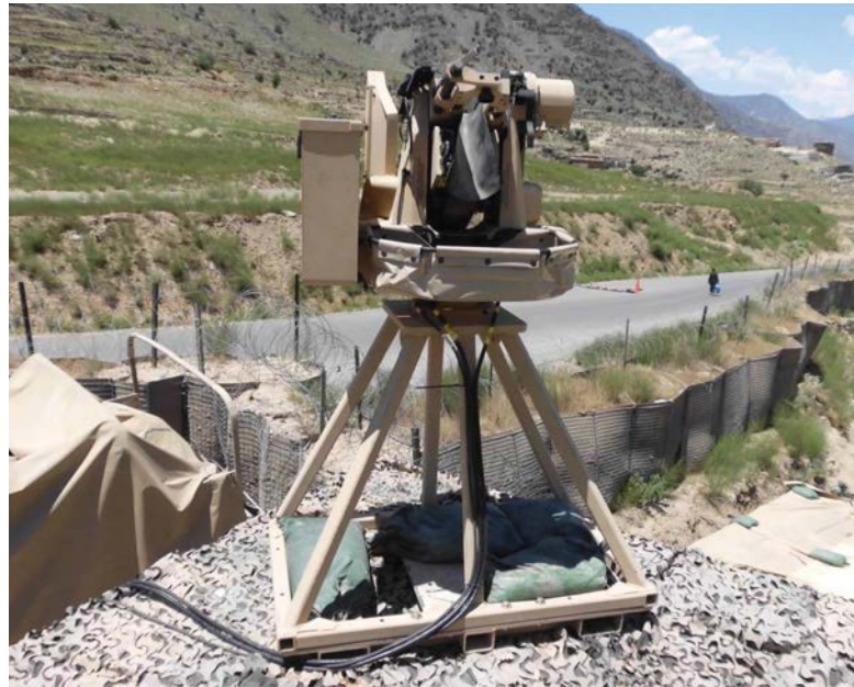
Common Remotely Operated Weapon Station systems are also mounted on towers at bases of operations in Afghanistan. They provide protection to the bases by enhancing their ability to detect the enemy and engage simultaneously if necessary. (U.S. Army photo)
