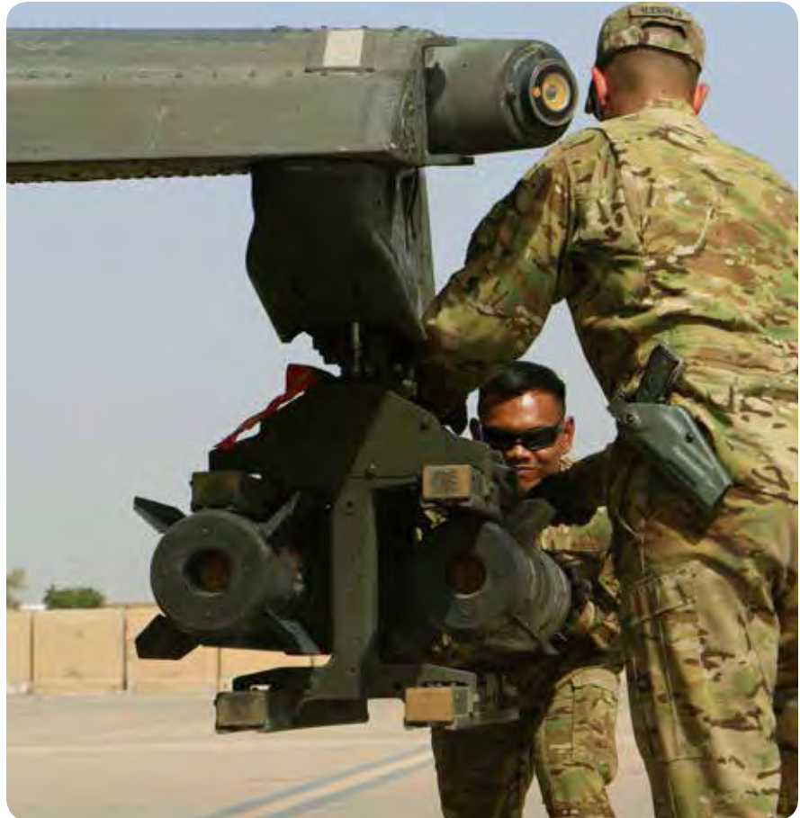
ABOVE: U.S. Army Pfc. Jazel Yadao, AH-64 Apache attack helicopter repairer, and U.S. Army Sgt. Sean Parker, Apache armament/electrical/avionic system repairer, both assigned to 1st Attack Reconnaissance Battalion, 10th Aviation Regiment, 10th Combat Aviation Brigade, slide a Hellfire missile into place on an Apache at Taji Airbase, Iraq. (U.S. Army photo by Sgt. 1st Class R.W. Lemmons IV)
