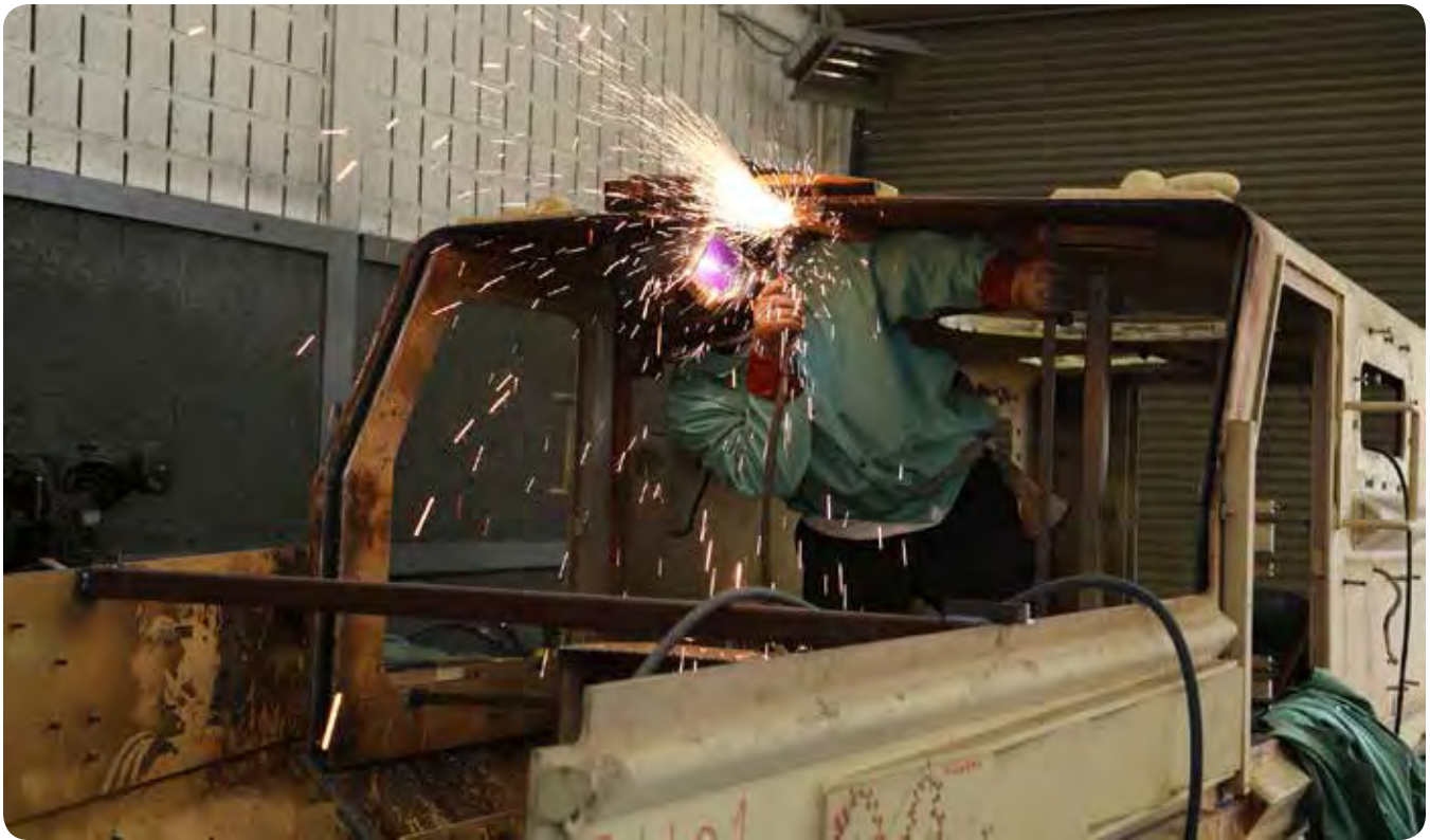
A Red River Army Depot team member conducts welding work inside the hull a Mine Resistant Ambush Protected Vehicle. The depot is capable to rebuild and repair each variant of the MRAP.
