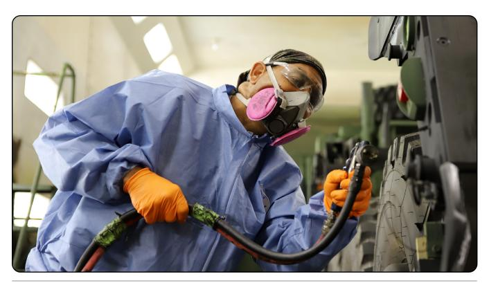
Jeff Porter, a painter at the Fort Stewart Maintenance Paint Booth, finishes applying camouflage paint to a Palletized Load System vehicle. Once the painting process is complete, the vehicle will be shipped over to Europe as part of the European Defensive Initiative. (U.S. Army photo by Sgt. 1st Class Corey Baltos)
