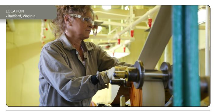
An employee rolling solventless propellant as a part of the propellant production process at RFAAP. (Courtesy photo)
