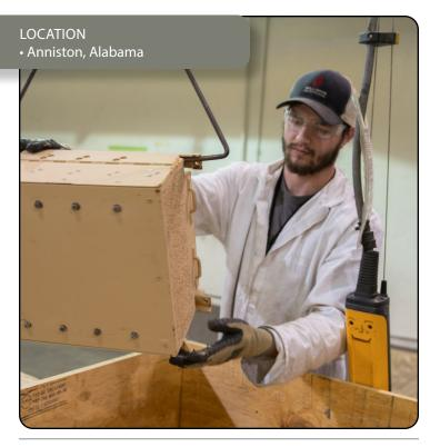
ABOVE: An ANMC employee inspects a reactive armor tile for usability. Tiles which can be repaired are cleaned, inspected again, fixed and painted. (U.S. Army Photo by Anniston Munitions Center) BELOW: An ANMC Munitions Division employee loads a 20-foot container of munitions for relocation to another site within the Joint Munitions Command Munitions enterprise. (U.S. Army photo by Mark Cleghorn)
