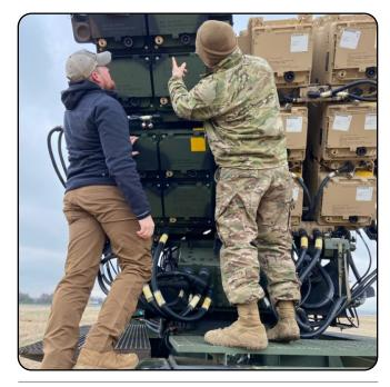
Kyle Battles, a Joint Munitions Command Quality Assurance Specialist (Ammunition Surveillance) expert, checks the humidity indicator on a Patriot surface-to-air missile system in Zagan Poland, recently (Courtesy photo)
