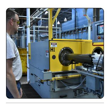
A Quad City Cartridge Case Facility employee loads obsolete MK9 cartridge cases as a part of the retrofitting process to recycle old cartridge cases into modernized MK109 versions to accommodate new propellant for the Navy. (U.S. Army photo by Dori Whipple)
