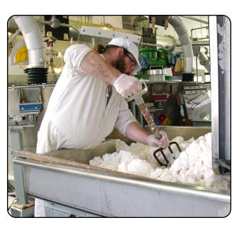
A contractor employee for Holston Army Ammunition Plant works with coated composition C-4 before it's packaged and shipped to the customer. (Courtesy photo)
