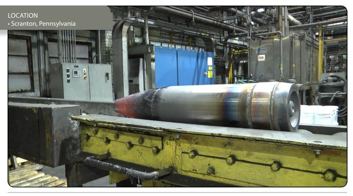
Projectile at SCAAP moves on a conveyor to the heat-treating process after completion of the nosing process. Nosing is the process where the open end of the cylindrical parts are formed into the roundly-tapered ogive. (Courtesy photo)
