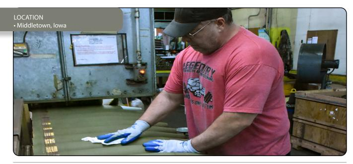
A contractor employee at IAAAP cleans 155mm artillery rounds as a step in the load, assemble, pack process. (Courtesy photo)
