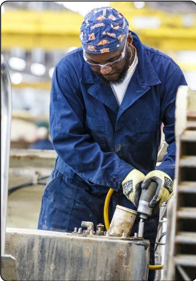
Tyrone Garrett removes the rear sending unit from a rear fuel cell on a M1A2 in Anniston Army Depot’s Combat Vehicle Repair Facility. (U.S. Army photo by Mark Clegghorn)
