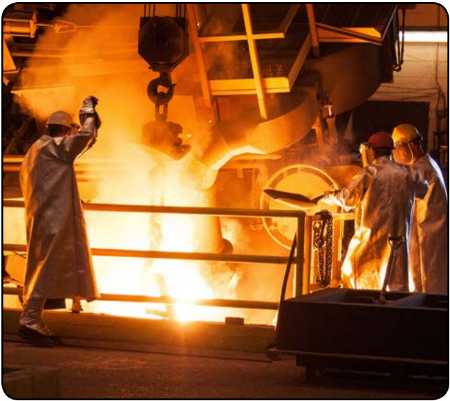
Rock Island Arsenal-Joint Manufacturing and Technology Center foundry employees conducted a test pour to prove out a new pour basin for the M777 howitzer muzzle break at Rock Island Arsenal, Illinois. The new muzzle break casting is designed by the University of Iowa. In addition to the muzzle break, pours for test plates used to certify weld processes on the muzzle break and test bars used to verify heat-treat processes were completed. This effort is working to improve muzzle break pours, producing the finest products for the warfighter. (U.S. Army photo by Debralee Best)
