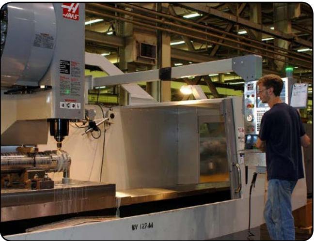
A Watervliet machinist performs a vertical milling operation on a cannon. (U.S. Army photo by William Martin)
