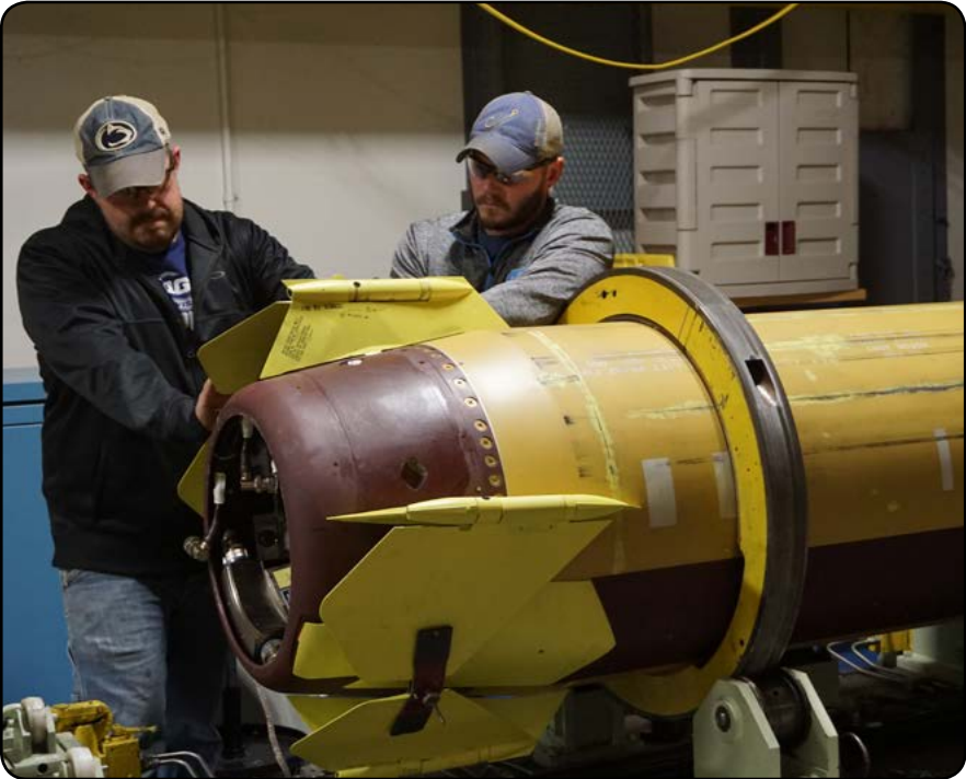
Letterkenny Munitions Center (LEMC) technicians prep an Army Tactical Missile Systems for control section removal. LEMC is the U.S. Army's Center of Industrial and Technical Excellence for the Multiple Launch Rocket System Family of Munitions. (U.S. Army photo by Natasia Kenosky)
