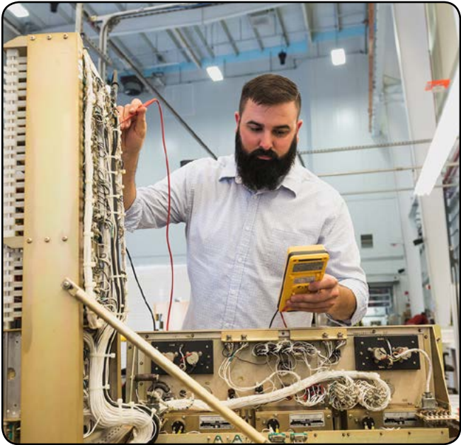
Electronics Mechanic Patrick Barrett performs electrical troubleshooting and alignment on a tracking control for the AN/MPS-T1 Band Simulator System. Tobyhanna Army Depot has been performing programmed depot maintenance on the band simulator system for more than 15 years. It takes 12 employees nearly two years to repair the critical Air Force system. The primary purpose of the radar set is to provide a realistic surface-to-air missile control radar environment, which can be used to train, test, and evaluate aircrew performance. Barrett works in the C4ISR Directorate's Single Threat Systems Branch. (U.S. Army photo by Tom Robbins)
