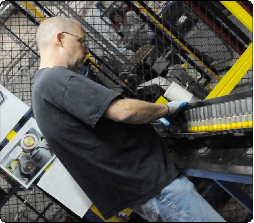
An operating contractor employee at Iowa Army Ammunition Plant prepares linked 40mm grenade ammunition to be packed into an ammunition box. (U.S. Army photo by Tony Lopez)
