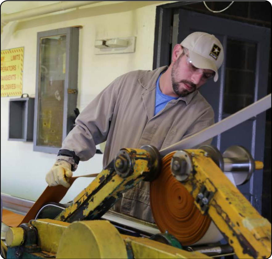
A Radford Army Ammunition Plant employee rolls solventless propellant as a part of the production process. (U.S. Army photo)
