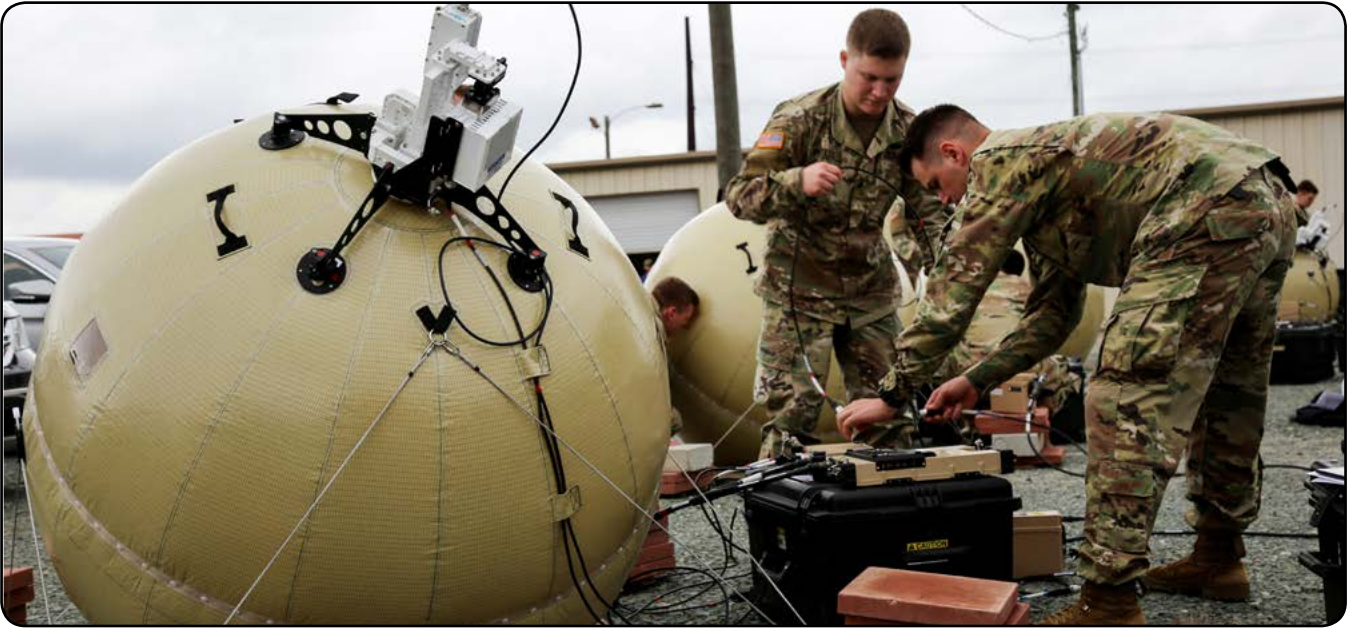
Once on the ground and an airfield is seized, Soldiers can rapidly set up their inflatable Transportable Tactical Command Communications, or T2C2 satellite system, and retain continuity of mission command during the initial phase of the operation. Later in the mission, when follow-on forces fly in larger network assets, commanders can extend the battlespace using T2C2 to support company-size forward operating bases and special team-size elements that need an easily transportable network capability at the tactical edge. (U.S. Army photo by Amy Walker)
