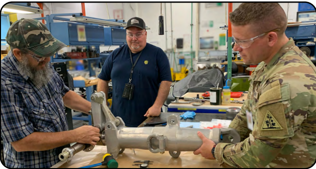
LEFT: CCAD Rotor Control Supervisor Rodney Helms, assists SSG Pete Johnson (right), Aviation Hydraulics Mechanic with the 1109th TASM CT ARNG, assemble a forward shop strut landing gear for a CH-47 Chinook helicopter at the Corpus Christi Army Depot as Rotor Control Mechanic Gonzalo Villarreal, Jr. observes. (Courtesy photo)
