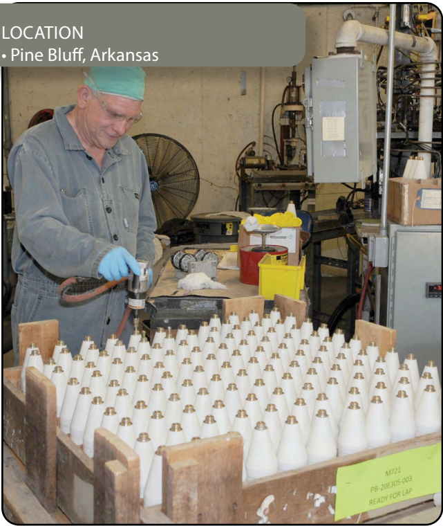
An ammunition production worker removes a bolt from an illumination round on the 60mm body-load production line. (U.S. Army photo by Hugh Morgan)
