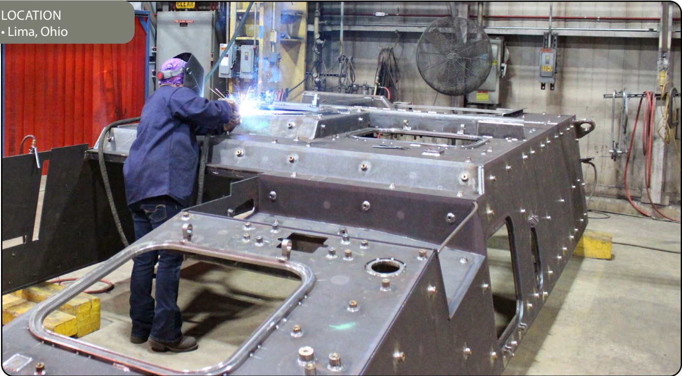
A welder fabricates the upper structure of a Stryker Combat Vehicle at the Joint Systems Manufacturing Center-Lima. (U.S. Army photo by Brian Hahn)
