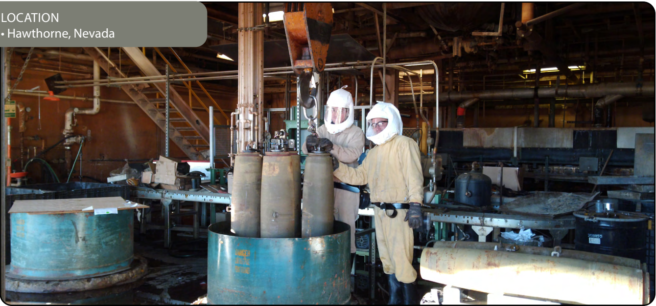
Employees at Hawthorne Army Depot lower obsolete ammunition stockpile items into a belt flaker as part of the decontamination and demilitarization process at HWAD. (U.S. Army photo by Hawthorne Army Depot)
