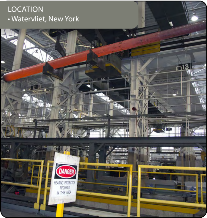
A 155mm Howitzer tube being moved from the Watervliet Arsenal's rotary forge to a cooling area. The forging operation, which heats tubes up to nearly 2,000 degrees, is the first critical machining operation performed on large caliber Howitzer. (Courtesy photo)
