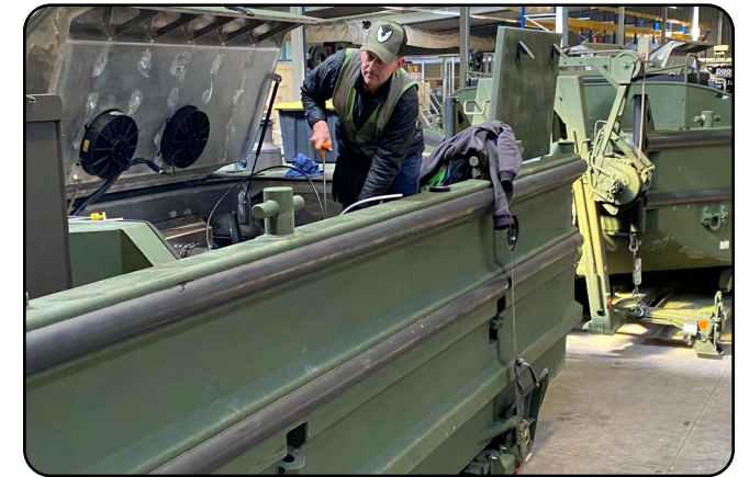
Davy Aerts, a heavy wheeled vehicle mechanic, adjusts the engine oil level on an M30 Bridge Erection Boat. The workforce at the Army Prepositioned Stocks-2 Zutendaal worksite in Belgium consists of U.S. personnel and Belgium local nationals. They've been tasked with preparing nearly 4,700 APS-2 vehicles and equipment pieces in support of U.S. Soldiers deployed to Europe. The boat is part of a float bridge set, several of which are stored and maintained at APS-2 Zutendaal. (U.S. Army photo by Cameron Porter)
