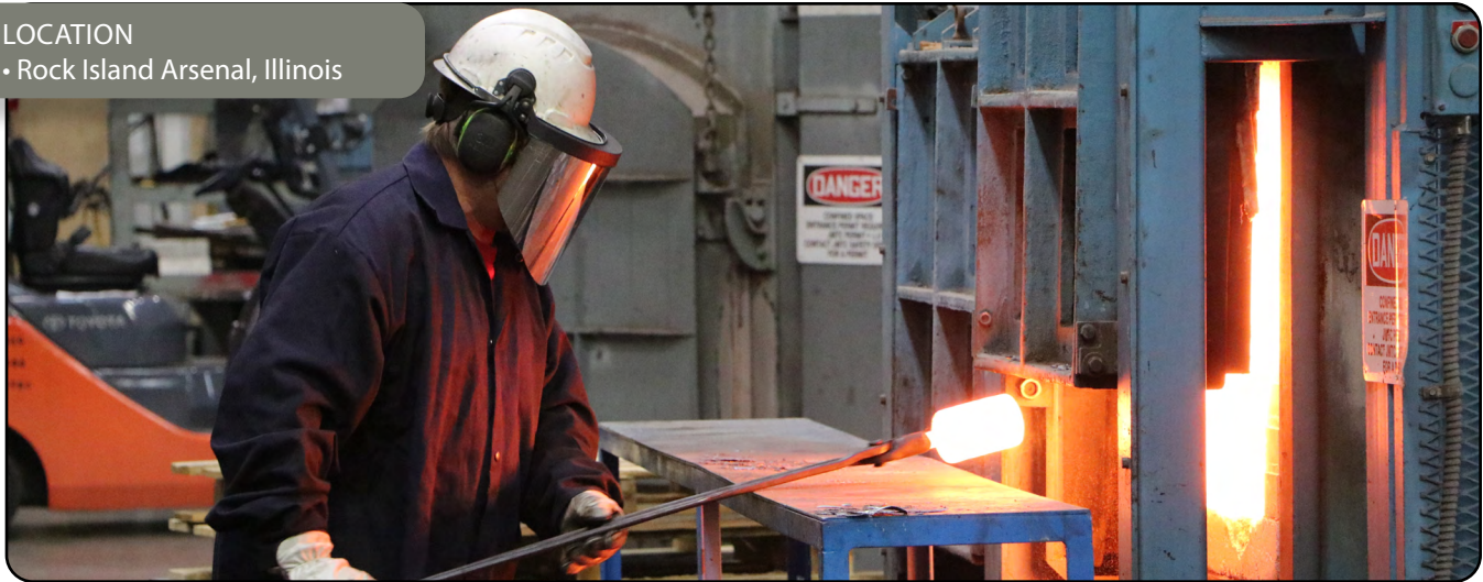
Temperature is key when working with metal. This Rock Island Arsenal-Joint Manufacturing and Technology Center artisan pulls metal out of a furnace to cool before it flattened by a hammer. RIA-JMTC is a vertically-integrated metal manufacturer capable of taking raw material and bringing it to a finished product all under one roof. Rock Island Arsenal-Joint Manufacturing and Technology Center develops, manufactures and delivers readiness to the warfighter through both conventional and advanced manufacturing processes.(U.S. Army photo by Hayley Smith)
