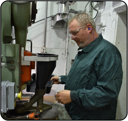
MODERNIZATION: An explosives handler sets up an updated Stokes rotary press to begin a new project. Recently a Crane Army Ammunition Activity engineering team retrofitted equipment controls on the press as part of Crane Army's ongoing modernization effort. (U.S. Army photo by Christy Carroll)
