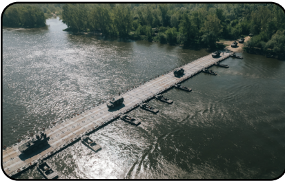
BACK COVER: A float ribbon bridge system from the Army Prepositioned Stocks-2 worksite in Zutendaal, Belgium, is used by U.S., Polish, French and Swedish military forces to cross the Vistula River during DEFENDER-Europe 22, May 13. The float bridge is part of the 405th Army Field Support Brigade's APS-2 program. This was the first time a float bridge system from the Zutendaal APS-2 site was transported to Poland and used during a DEFENDER-Europe exercise. (Photo by Michal Czornij)
