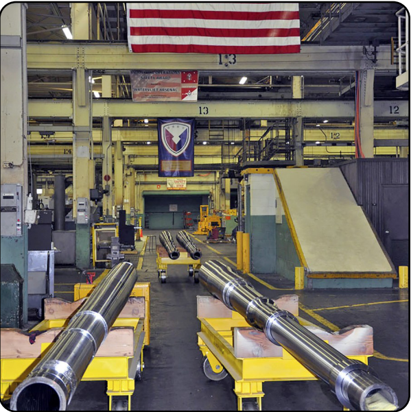
A 155mm Howitzer tube being moved from the Watervliet Arsenal's rotary forge to a cooling area. The forging operation, which heats tubes up to nearly 2,000 degrees, is the first critical machining operation performed on large caliber Howitzer. (Courtesy photo)
