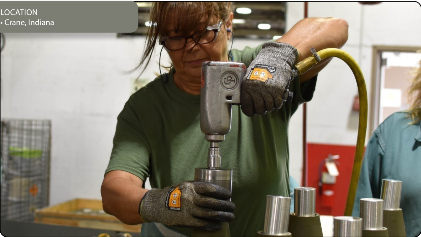
An explosives handler at Crane Army Ammunition Activity removes the expulsion cup on a 155mm. (U.S. Army photo by Christy Carroll)
