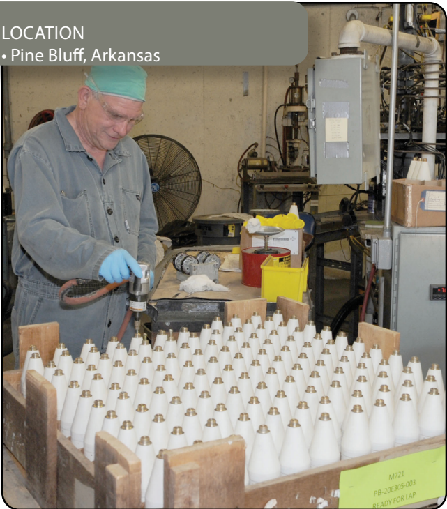
An ammunition production removes a bolt from an illumination round on the 60mm body-load production line. (U.S. Army photo by Hugh Morgan)
