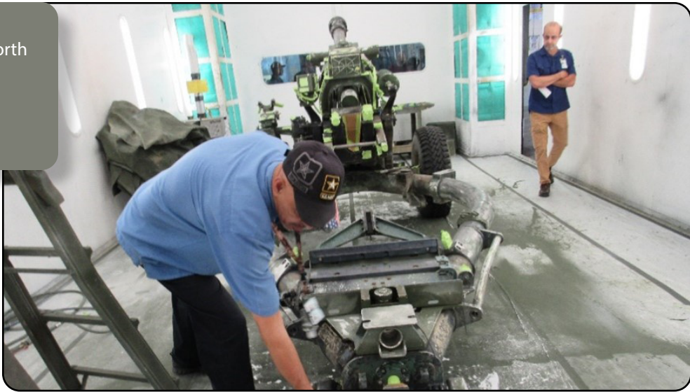
Michael Dorsey, a Quality Assurance Inspector at the Fort Liberty Maintenance Paint Booth, verify preparation work prior to applying camouflage paint to a M119A2 Howitzer. Once the painting process is complete, the weapon system will be shipped back to the unit to support sustainment of the Fires Brigade in support of the immediate response force mission initiative. (Courtesy photo)
