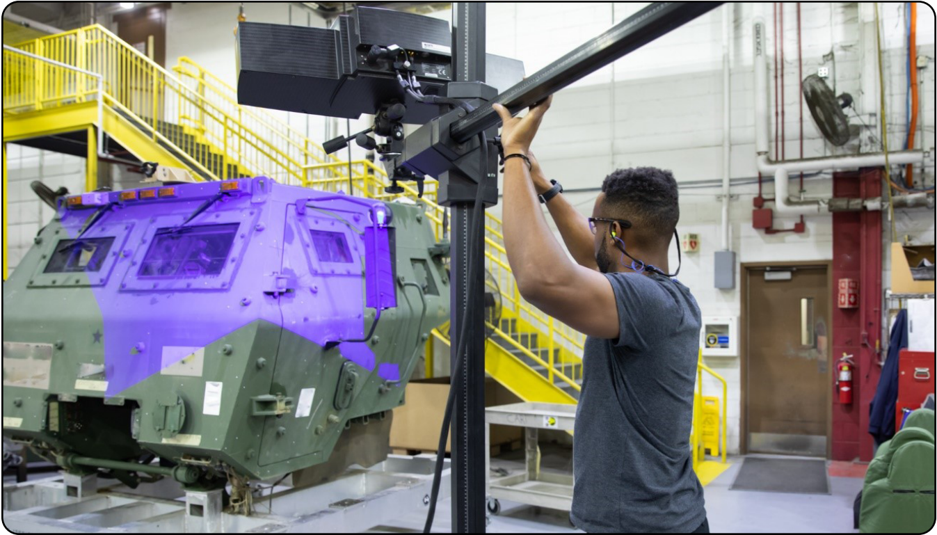
Kennon Matthews, lead metrologist, Letterkenny Army Depot, performs blue light scanning on a High Mobility Artillery Rocket System cab March 14, 2022. Blue-light scanning technology was initially acquired to generate surface measurement analyses of turrets for the Extended Range Cannon Artillery program at Letterkenny. (U.S. Army photo by Pam Goodhart)
