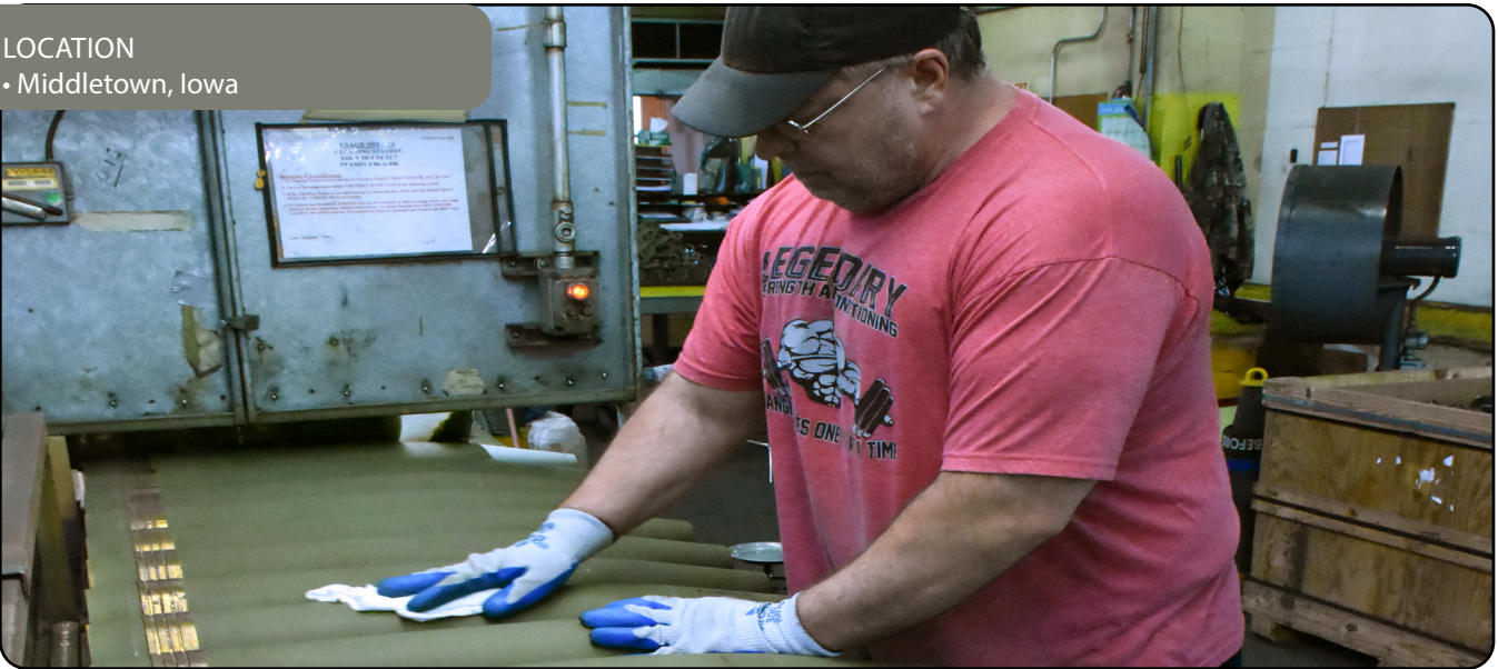
A contractor employee at IAAAP cleans 155mm artillery rounds as a step in the load, assemble, pack process. (Courtesy photo)
