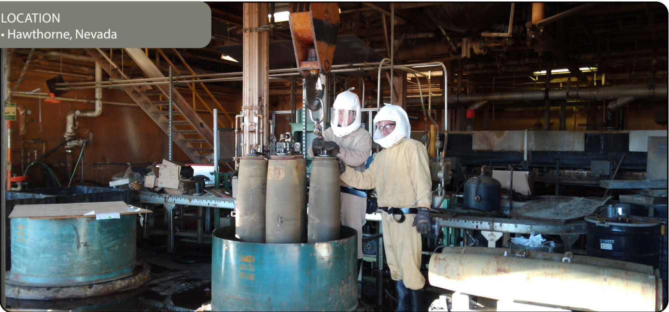
Employees at Hawthorne Army Depot lower obsolete ammunition stockpile items into a belt flaker as a part of the decontamination and demilitarization process. (U.S. Army photo by Hawthorne Army Depot)
