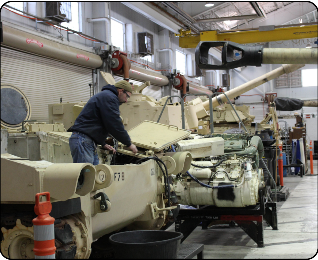
Missile and Fires Division employee performing engine maintenance on M109A6 Paladin Howitzer. (Courtesy photo)
