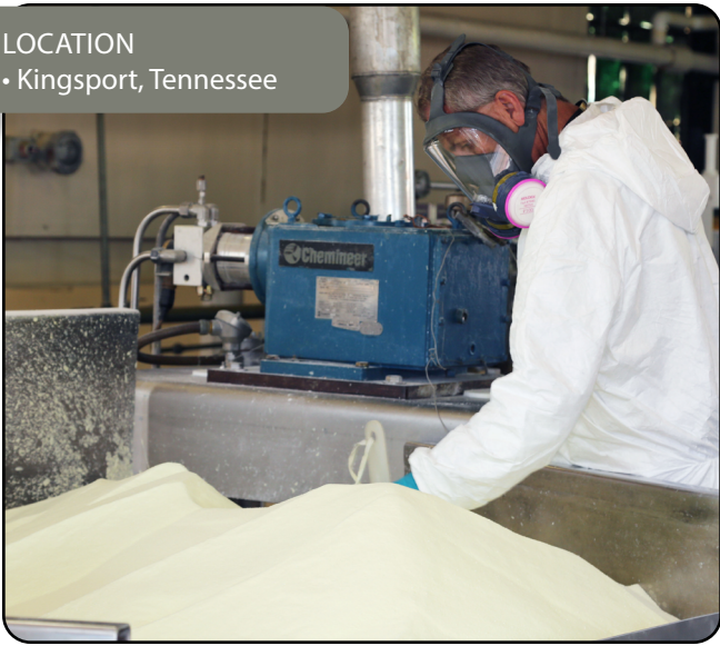
A contractor employee for Holston Army Ammunition Plant prepares explosives on a charging table to be bagged and placed into a drum. (Courtesy photo)
