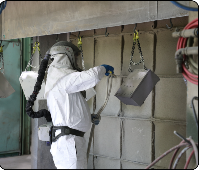
Blue Grass Army Depot employee uses modernized ventilation system while refurbishing reactive armored tiles for future military use. (U.S. Army photo by Dori Whipple)
