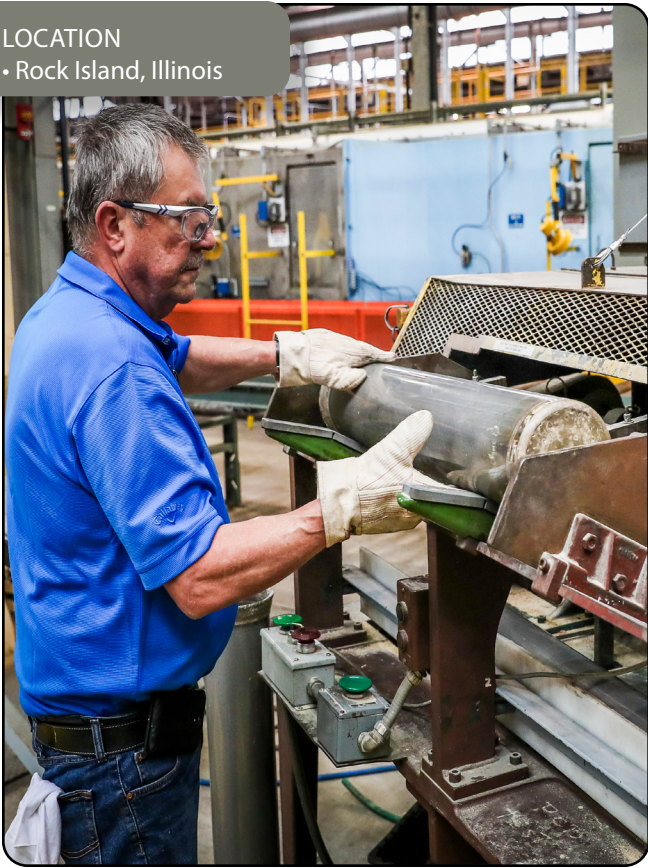
A technician loads a cartridge case during the press operations into a trimming machine that will adjust the length to correctly move it to the next pressing operation at QCCCF at the U.S. Army's Rock Island Arsenal, Rock Island, Illinois. (U.S. Navy photo by Matthew Poynor)
