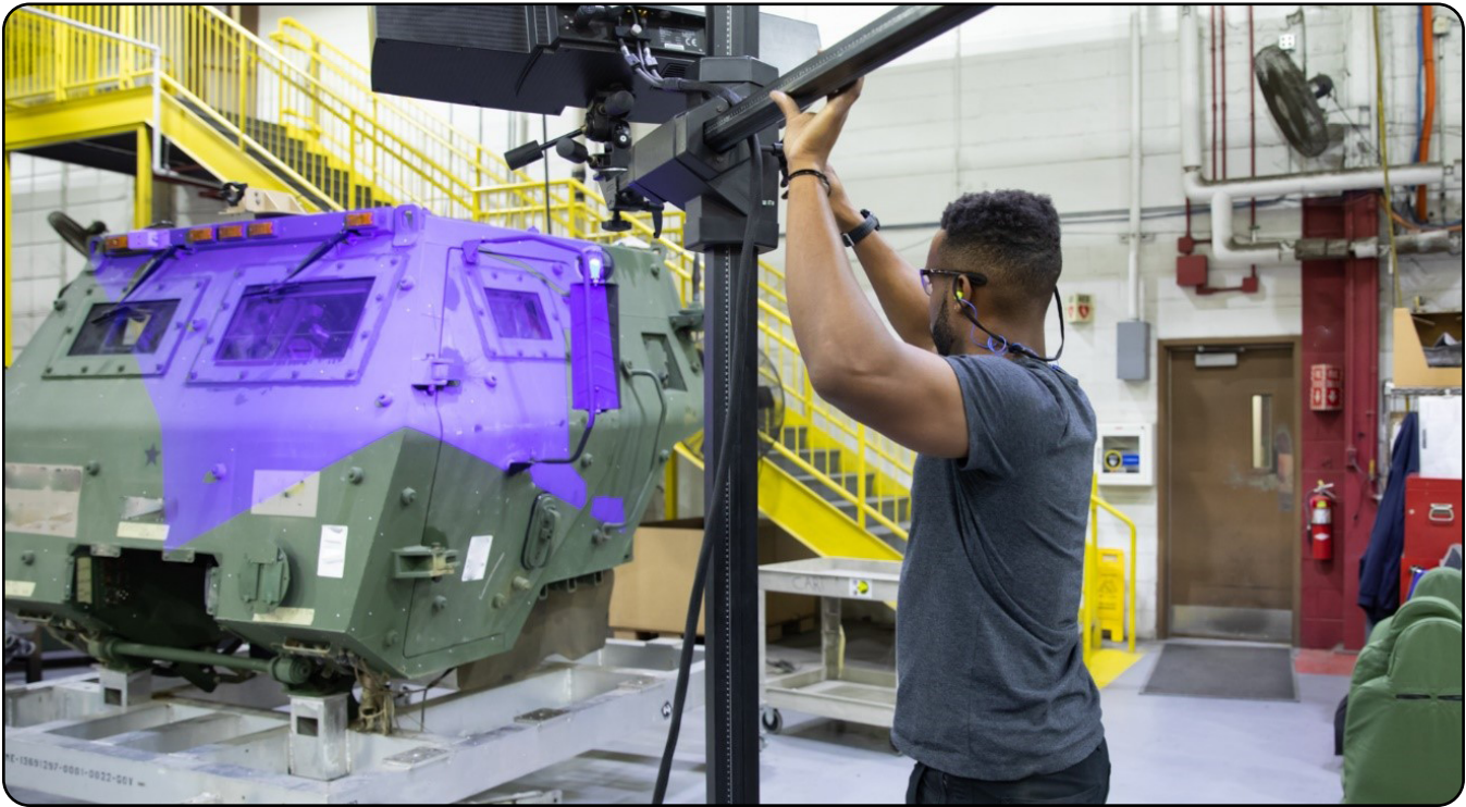
Kennon Matthews, lead metrologist, Letterkenny Army Depot, performs blue light scanning on a High Mobility Artillery Rocket System cab March 14, 2022. Blue-light scanning technology was initially acquired to generate surface measurement analyses of turrets for the Extended Range Cannon Artillery program at Letterkenny. (U.S. Army photo by Pam Goodhart)
