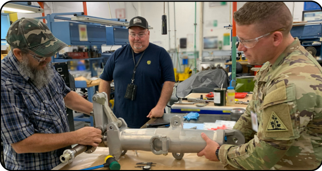
LEFT: CCAD Rotor Control Supervisor Rodney Helms, assists SSG Pete Johnson (right), Aviation Hydraulics Mechanic with the 1109th TASM CT ARNG, assemble a forward shop strut landing gear for a CH-47 Chinook helicopter at the Corpus Christi Army Depot as Rotor Control Mechanic Gonzalo Villarreal, Jr. observes. (Courtesy photo)
