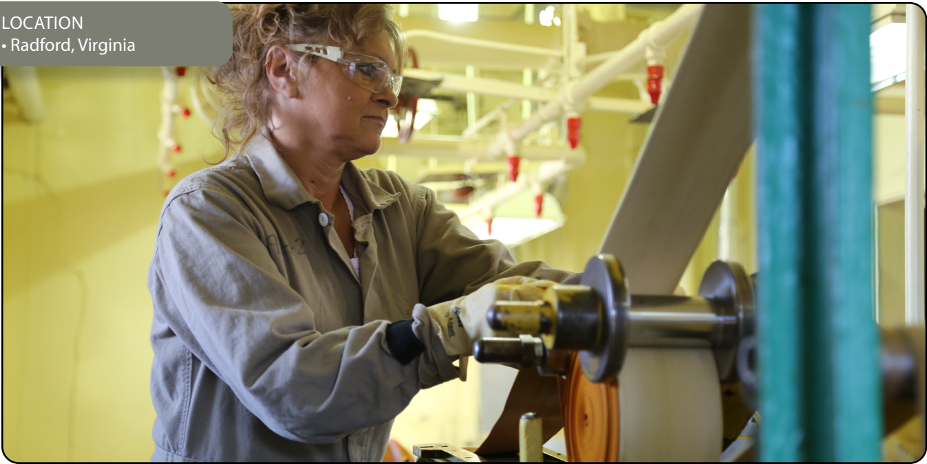
An employee rolling solventless propellant as a part of the propellant production process at RFAAP. (Courtesy photo)
