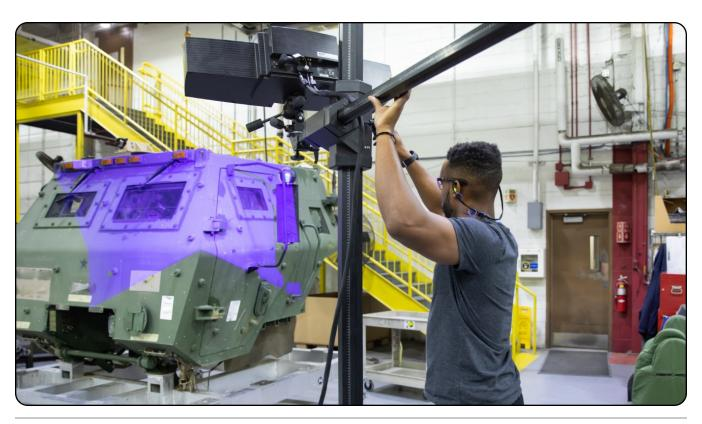
Kennon Matthews, lead metrologist, Letterkenny Army Depot, performs blue light scanning on a High Mobility Artillery Rocket System cab March 14, 2022. Blue-light scanning technology was initially acquired to generate surface measurement analyses of turrets for the Extended Range Cannon Artillery program at Letterkenny. (U.S. Army photo by Pam Goodhart)
