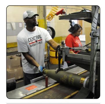
An employee at Iowa Army Ammunition Plant labels a 155mm artillery round on the artillery paint line (U.S. Army photo by Iowa Army Ammunition Plant)
