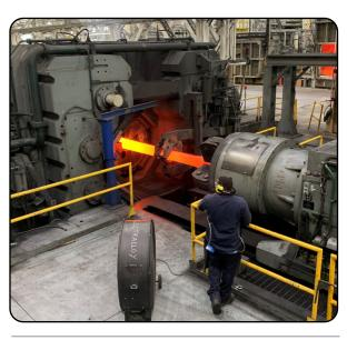
ABOVE: Watervliet Arsenal forge workers monitor a cannon tube being processed through the current rotary forge. Watervliet Arsenal plans to replace the forge with a new, more capable forge in 2026. (U.S. Army photo by Matthew Day)
