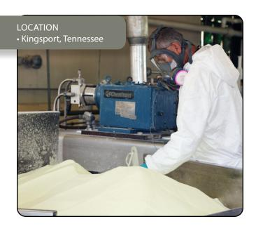
A contractor employee for Holston Army Ammunition Plant prepares explosives on a charging table to be bagged and placed into a drum. (Courtesy photo)
