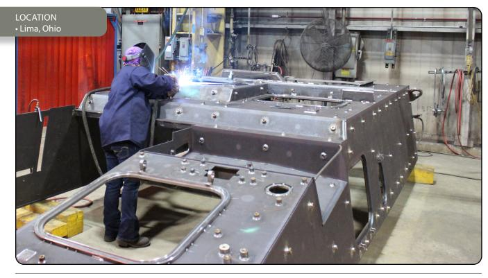
A welder fabricates the upper structure of a Stryker Combat Vehicle at the Joint Systems Manufacturing Center-Lima. (U.S. Army photo by Brian Hahn)
