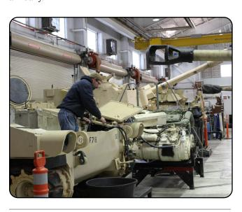
Missile and Fires Division employee performing engine maintenance on M109A6 Paladin Howitzer. (Courtesy photo)
