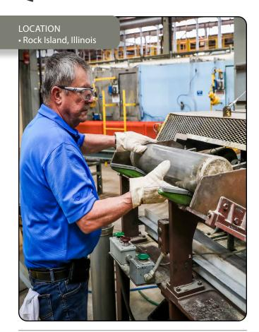
A technician loads a cartridge case during the press operations into a trimming machine that will adjust the length to correctly move it to the next pressing operation at QCCCF at the U.S. Army's Rock Island Arsenal, Rock Island, Illinois. (U.S. Navy photo by Matthew Poynor)
