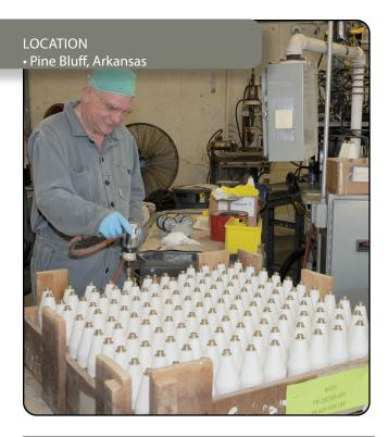
An ammunition production removes a bolt from an illumination round on the 60mm body-load production line. (U.S. Army photo by Hugh Morgan)
