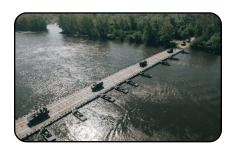
BACK COVER: A float ribbon bridge system from the Army Prepositioned Stocks-2 worksite in Zutendaal, Belgium, is used by U.S., Polish, French and Swedish military forces to cross the Vistula River during DEFENDER-Europe 22, May 13. The float bridge is part of the 405th Army Field Support Brigade's APS-2 program. This was the first time a float bridge system from the Zutendaal APS-2 site was transported to Poland and used during a DEFENDER-Europe exercise. (Photo by Michał Czornij)
