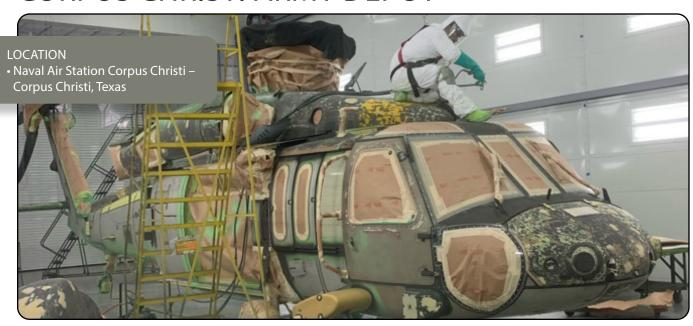
A Corpus Christi Army Depot painter journeyman applies the new "Class N" primer undercoat to the first Army Black Hawk helicopter. The process removes heavy metals from primer operations during aircraft maintenance. CCAD leads the way in implementing controls and protections for safer environments in depots and in the field where Soldiers and civilians perform maintenance. (Courtesy photo)
