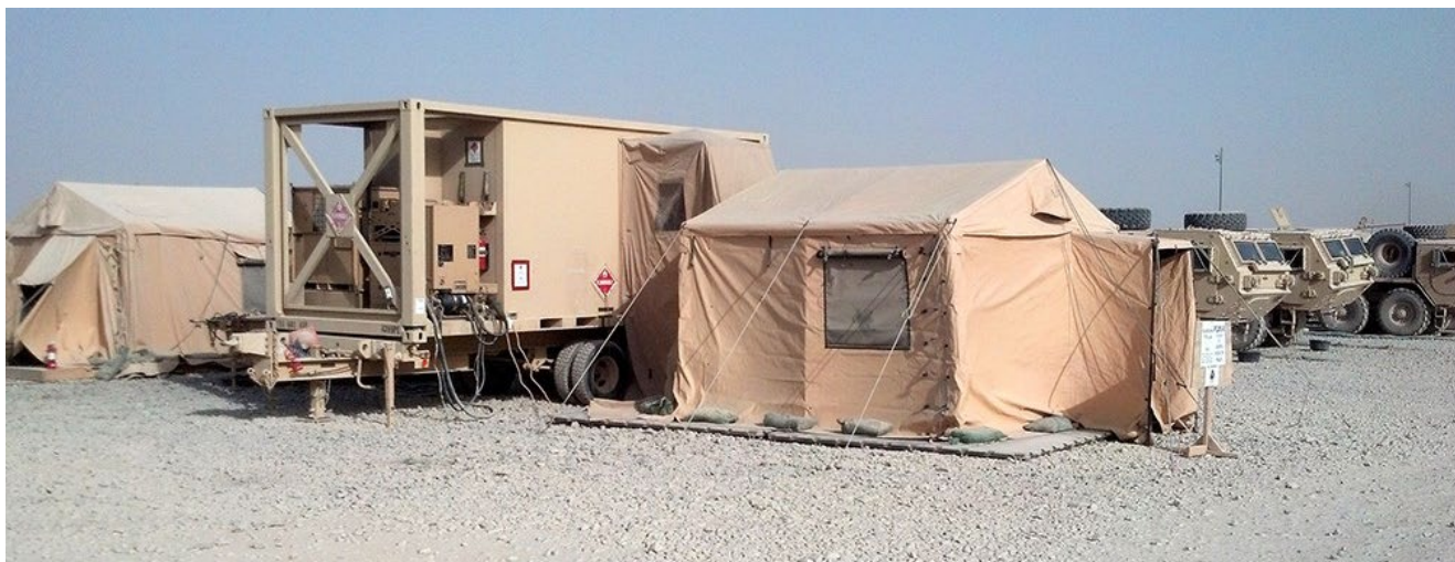
A Petroleum Quality Analysis System-Enhanced (PQAS-E) in Kandahar, Afghanistan. The PQAS-E is a complete automated petroleum laboratory capable of performing test procedures associated with the Army's quality surveillance mission on kerosene-based and military mobility fuels (U.S. Army photo by Sgt. George W. Slaughter).
